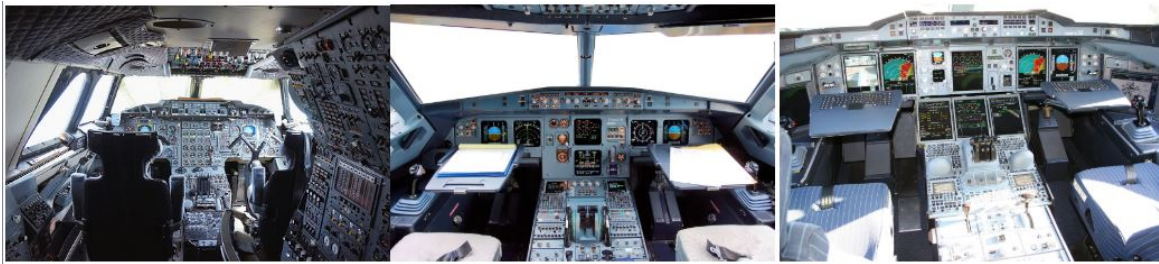
Figure 2. From left to right: Concorde's analog cockpit; glass cockpit in the A320; interactive cockpit in the A380 [4]
