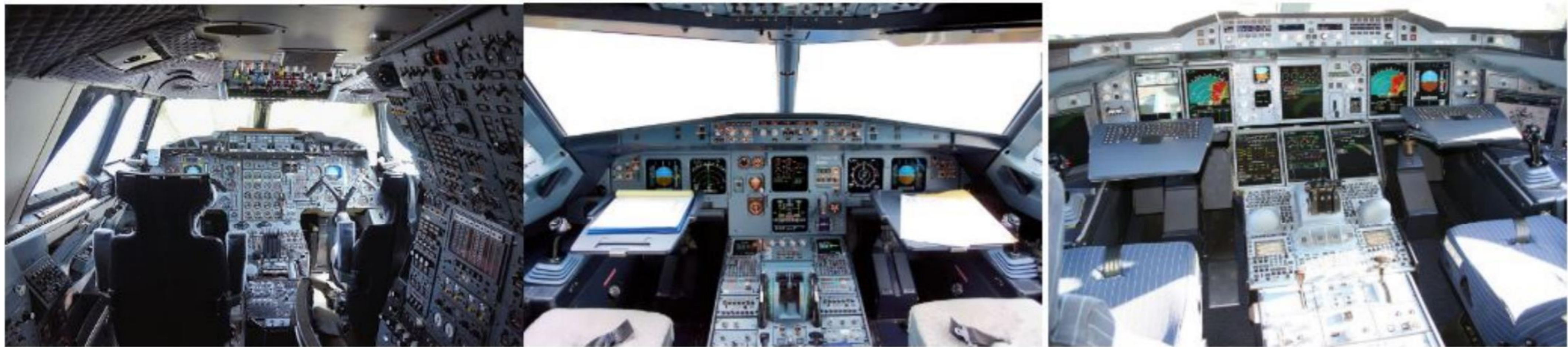
From left to right: Concorde's analog cockpit; glass cockpit in the A320; interactive cockpit in the A380
